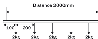
Track maximum loadings for single and three circuit
